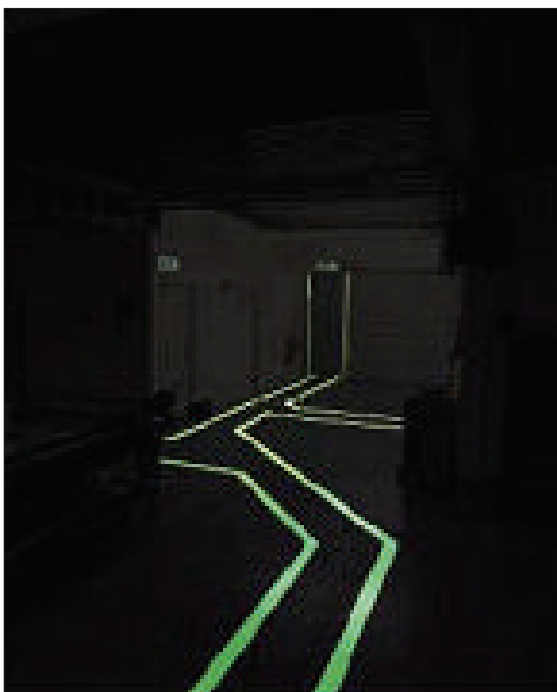
Figure 60: A 'way-guidance' system
