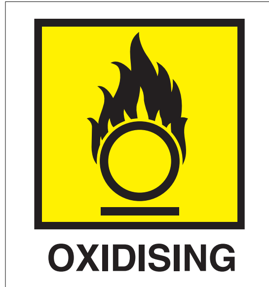
Figure 4: Label on oxidising materials
