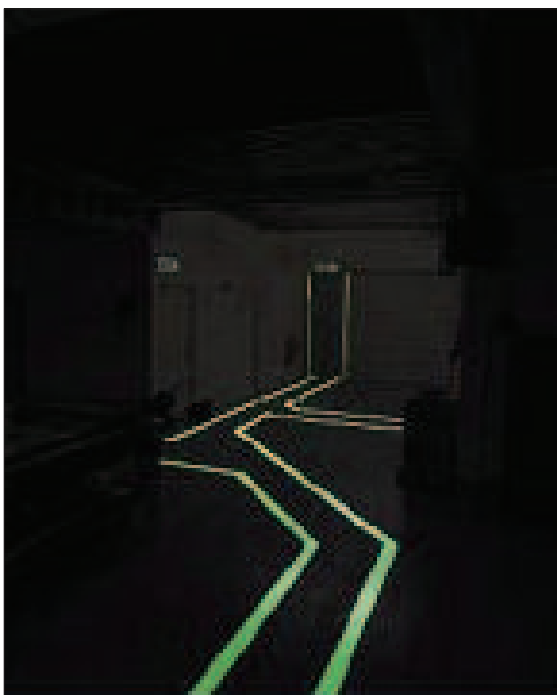
Figure 52: A 'way-guidance' system
