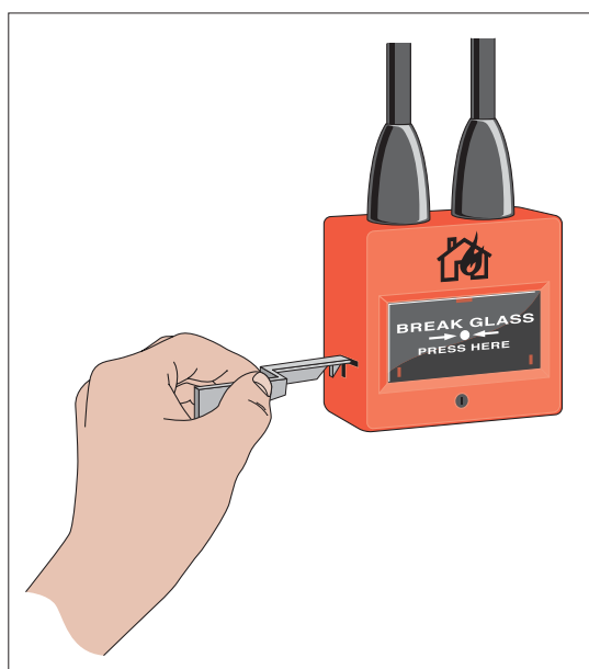
Figure 4: Sketch of fire alarm frangible cover break
